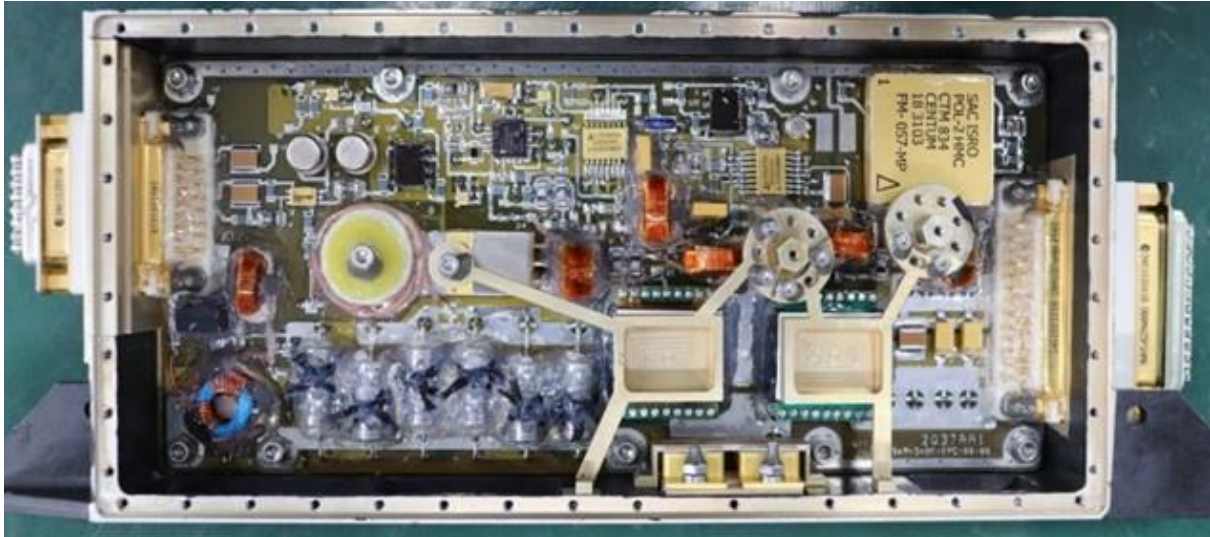
100W EPC with HMC based POL (NISAR)
