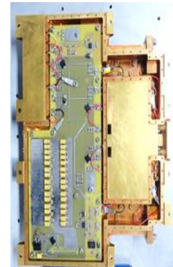
Integrated RF System Frequency Generator, Novel Spatial Combiner Receiver and Cavity Filter 350 X-Band SSPA
