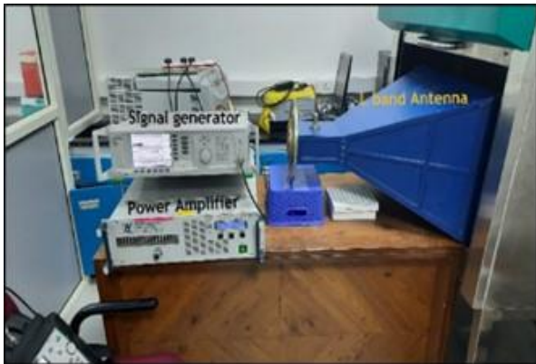
Experimental test setup using Satcom subsystems to validate the concept of viral fragmentation upon microwave exposure at its natural frequency.
