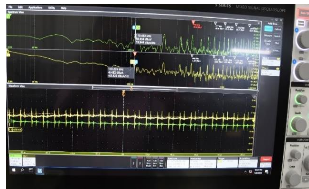
Fig 3b: Lower ripple when AEF enabled
