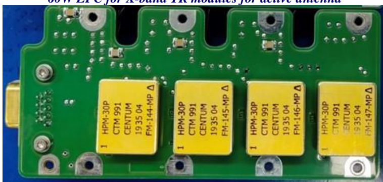
4 channel Pulse modulator using HMCs for active antenna
