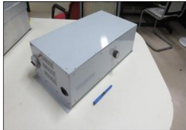
Miniaturized device prototype developed by SAC/SRO for corona virus fragmentation using microwave radiation.
