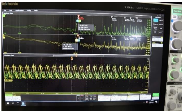
Fig 3a: Higher ripple when AEF disabled
